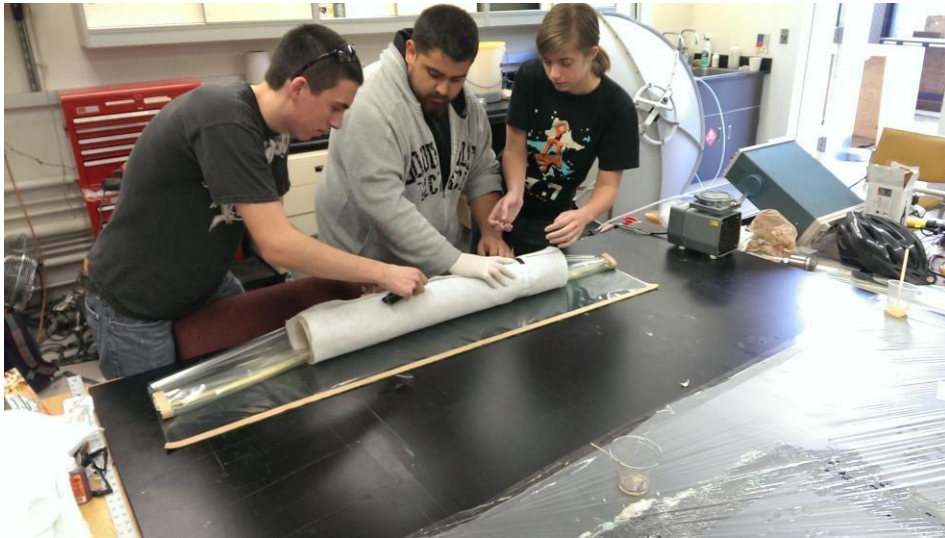
Figure 6: Vacuum Bagging a Cardboard Tube
