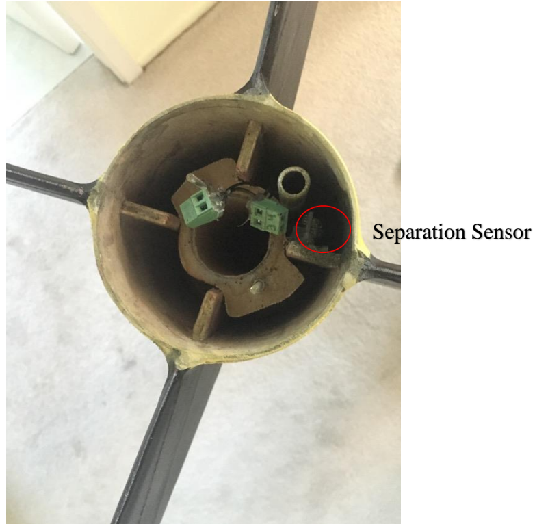
Figure 10. Connection Terminals for Separation and Ignition Charge, and Separation Sensor.
